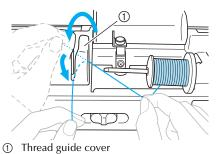
Pass the thread under the thread guide plate, and then pull it to the right.
